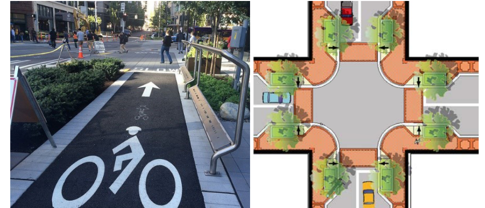
PEDESTRIAN FRIENDLY VEHICULAR USE AREA. IMAGES DEPICT: BICYCLE WAITING AREA AT AN INTERSECTION & TIGHTER INTERSECTIONS WITH BULB-OUTS
